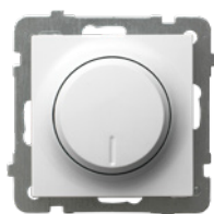
ŁP-8GAL2/m/00 2007 Universal dimmer load: GLS – 10-250W, CFL – 5-75W LED – 0-100W functions: electronic switch, "time to bed"
