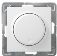
ŁP-8Y/m/00 1011 Push-turn dimmer adapted to incandescent and halogen loading, load 40-400W
