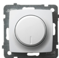
ŁP-8SL2/m/00 1574 Universal dimmer load: GLS - 10-250W, CFL - 5-75W, LED - 0-100W functions: electronic switch, "time to bed"
