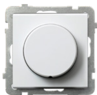
ŁP-8RL2/m/00 Universal dimmer load: GLS – 10-250W, CFL – 5-75W LED – 0-100W functions: electronic switch, “time to bed”
