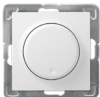
ŁP-8YL2/m/00 2005 Universal dimmer load: GLS – 10-250W, CFL – 5-75W LED – 0-100W functions: electronic switch, "time to bed"
